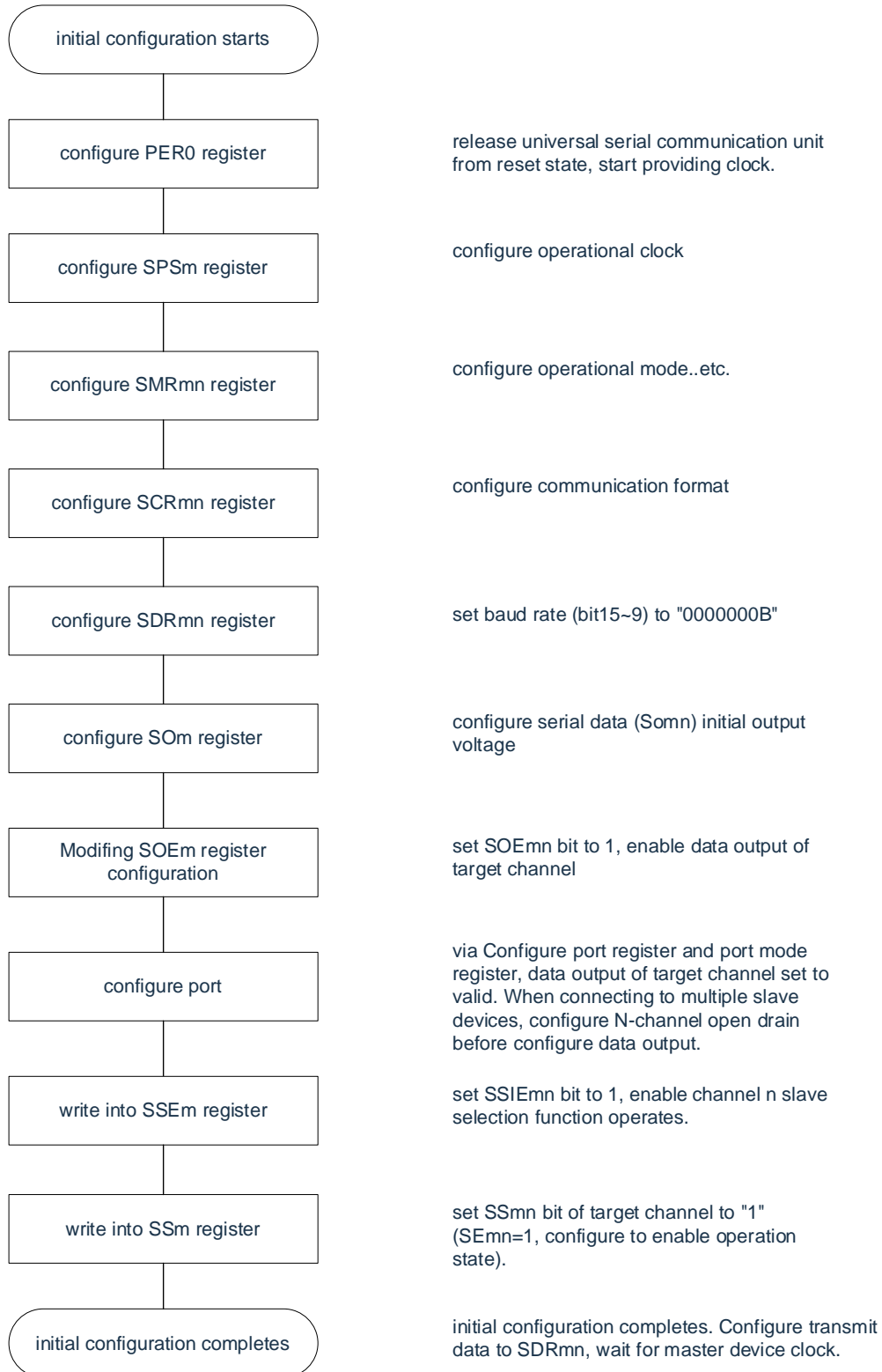
Figure16-88: Initial setup steps for slave sending and receiving
